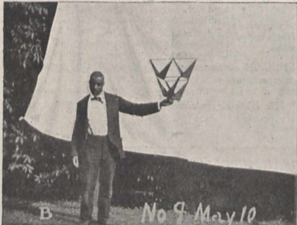
FIG. 2.—A Four-celled Tetrahedral Kite.
