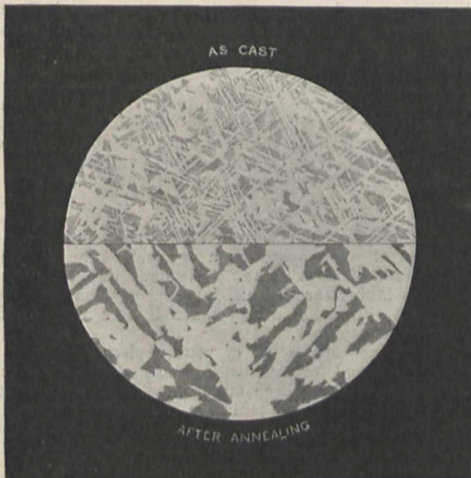
FIG. 1.—Research casting 541. Reduced from micrograph. Magnified 22 diameters.
