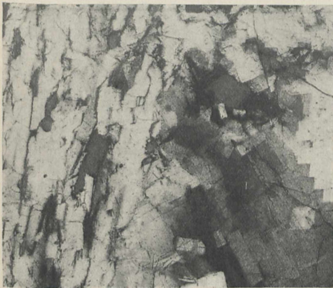
FIG. 1.—Tabular Crystals of Bytownite from Middle or Crucible. From "The Isomorphism and Thermal Properties of the Feldspars."
