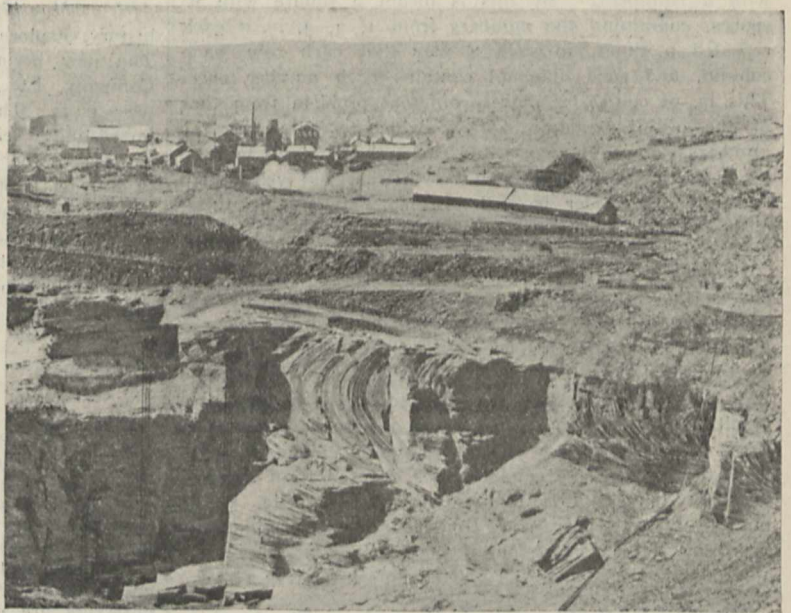
Old Bangor Slate Quarry, Bangor, Pa., S.S.W. End, showing the eroded overturned close syncline crossed by almost horizontal cleavage.
