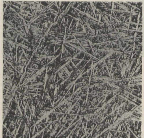
Quenched from 900° C. in water.
