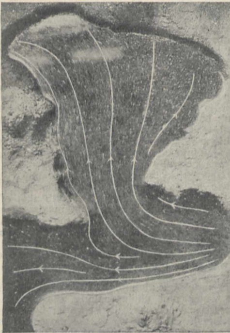
FIG. 2.—Model of Aomori Bay, showing stream lines of lateral oscillation: period 1'63 in model, representing 108 m. in the bay itself.
