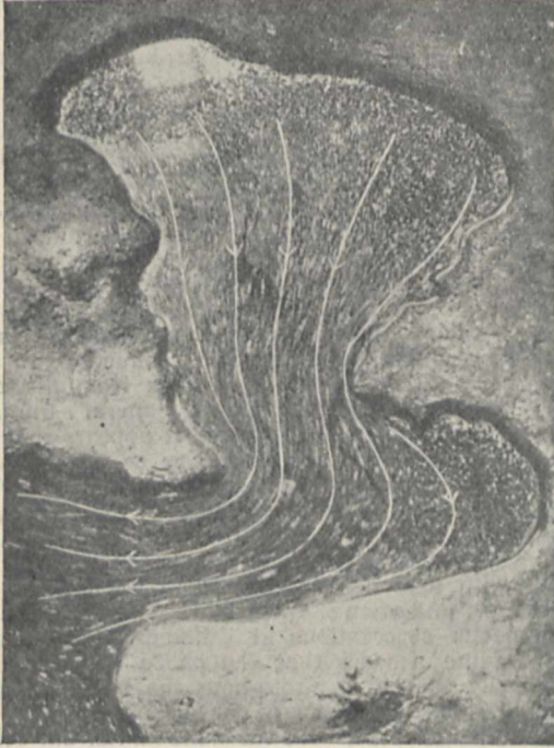
FIG. 1.—Model of Aomori Bay, showing stream lines of fundamental oscillation: period 4'453 in model, representing 303 m. in the bay itself.
