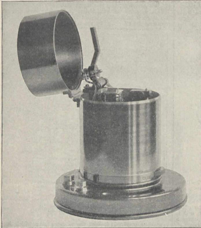
FIG. 6.—Telephone Relay in brass case with upper arm raised for cleaning the contents.
