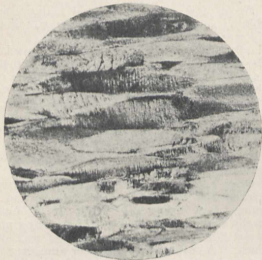
FIG. 1.—Structure of pure gold after being rolled. \times 11 .
