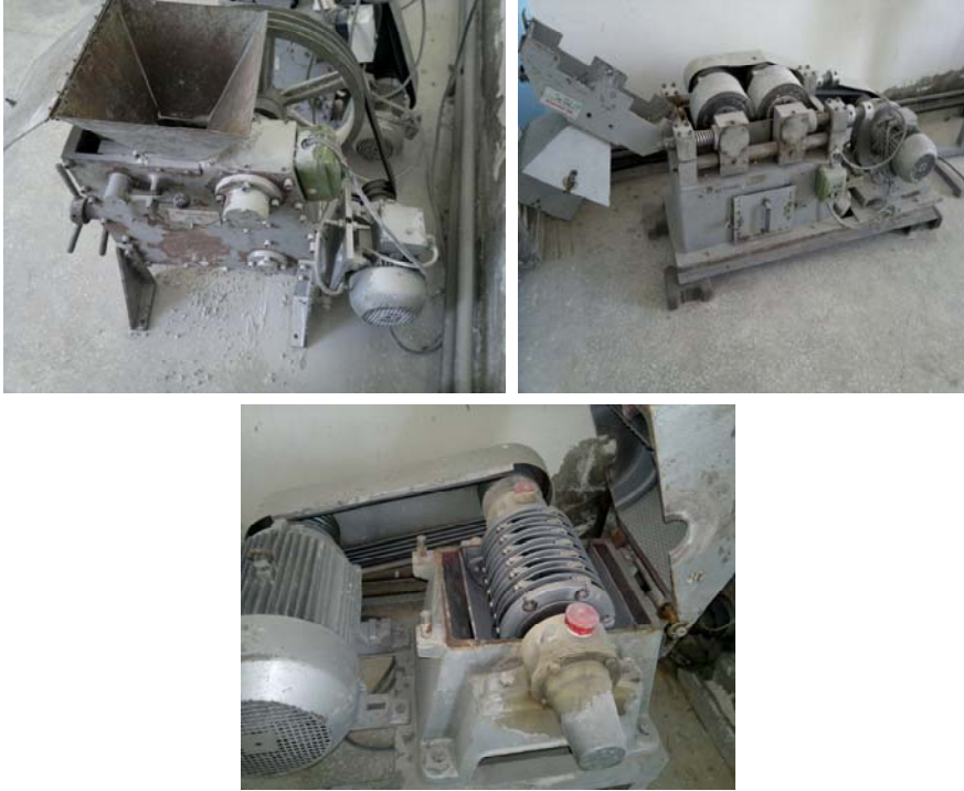
Fig. 2. Jaw, roller and hammer crushers used in the experiments
