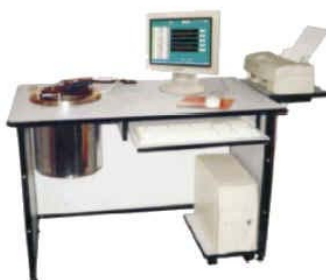
Figure 1. Calorimeter for determining heat of combustion
