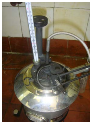
Fig.2. Stand to determine the flash point and the fire point of liquid fuels by the Marcusson method.
