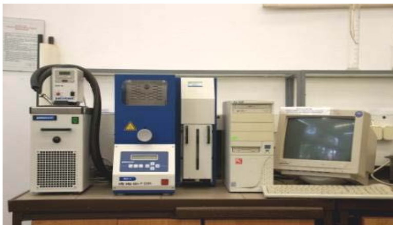
Fig 2. View of the apparatus for determining the fractional composition by distillation method at atmospheric pressure.
