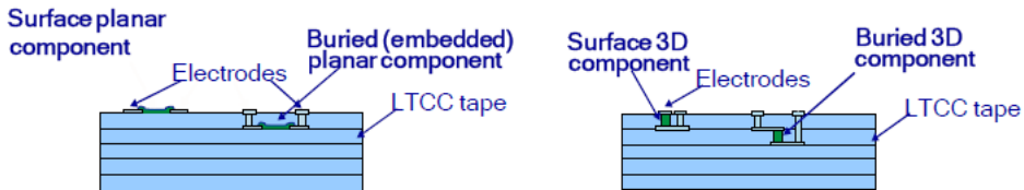
Fig. 2.12. Planar (2D) and 3-dimensional (3D) resistors
