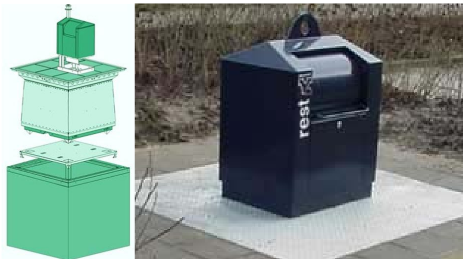
Figure 4-2. Schematic overview of a underground container (left) and the over ground insert unit (right) (Bammens 2010)
