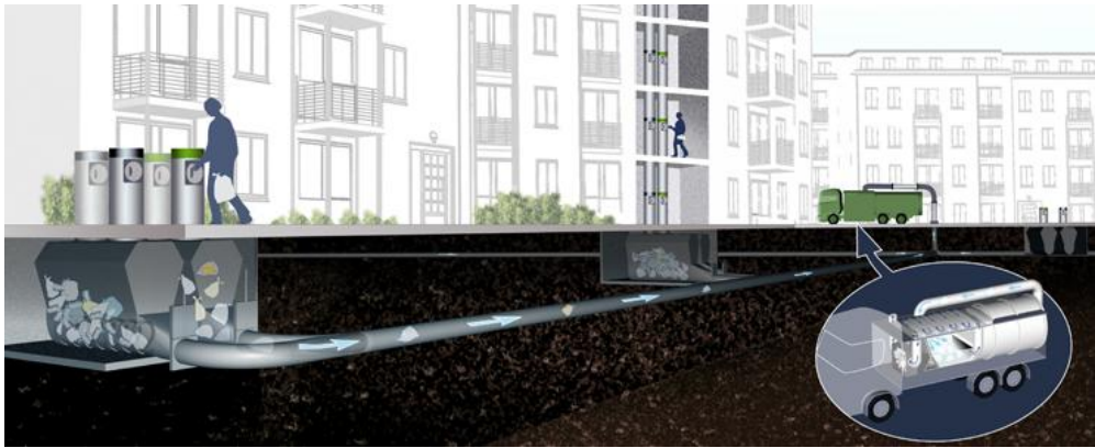
Figure 4-4. Waste sewer, mobile system (Envac 2010)
