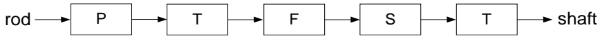
Fig. 34. Example of series reliability structure of a production system: P – saw, T – lathe, F – milling machine, S - grinding machine
