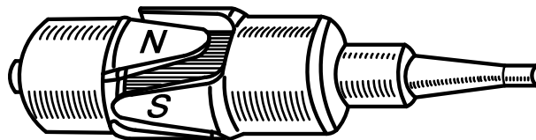
Fig. 6.9 The claw-shaped rotor of a brushless synchronous generator
