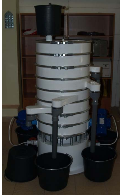
Fig. 2. A rolling-screw screen with a fraction receiver (Pocwiardowski and Wodzinski 2011b)
