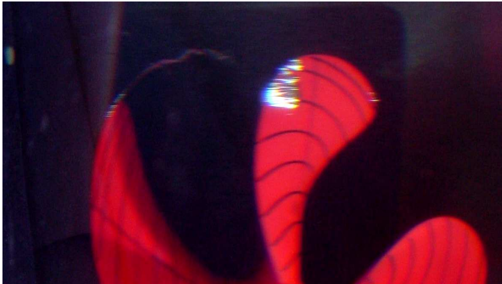
Fig. 3. Cavitating propeller tip vortex distorted by the rudder
