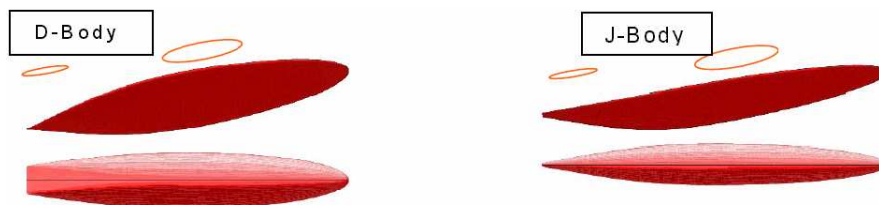
Fig. 2. D -Body and J -Body from aside and from above (location of main wing and horizontal tails is indicated (but these surfaces are not included in the grid))
