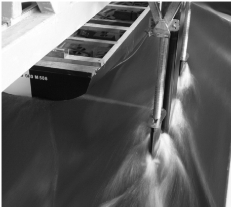
Fig. 5. PIV measurements on Navigator XXI model – the measurement stand
