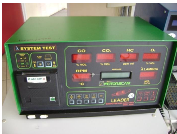
Rys. 4.17. Analizator spalin Mtorscan Leder 8000
