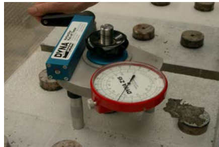
Fig. 7. Examination of bond layer adhesion to concrete surface
