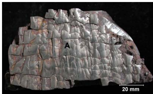
Fig. 2 [7]. Surface of CN-O padding weld after service (coal pulverizer). Three-layer padding weld, regenerated – 14500 working hours (5500 hrs after the last pad welding)
