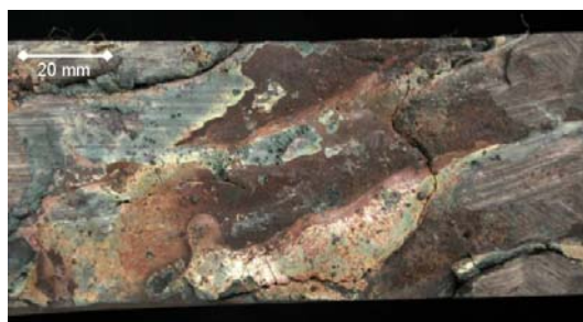
Fig. 3 [8]. Surface of the padding weld in ore crusher. The hardness at the padding weld surface: 591-613 HV_1 . Double-layer padding weld – the foundation layer was made with 3302 (E,C Termotec) electrode – applied in conditions of thermal shocks, loads and corrosion – the foundation hardness before hardening pad welding: ~200 HB and oxidation resistance to 600 °C. The surface layer was made with self-shielding electrode AN4923 (4923 E,C Termotec) of Ti, Mo and Cr. Although there is a foundation layer, the padding weld is highly cracked. On the surface there are visible weld penetration faults and cracks other than in Figure 1
