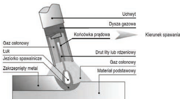
Rys. 1. Metoda spawania GMAW [7]
