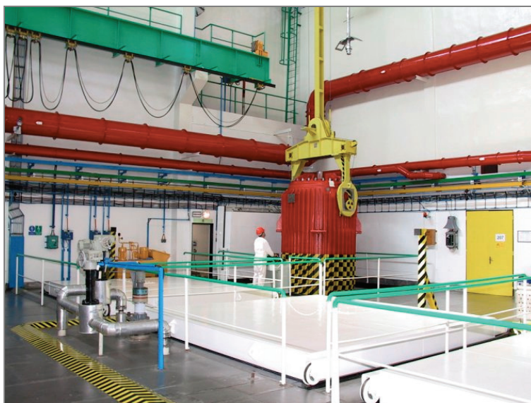
Fig. 3. Transport of casks TK C-30 [4]
