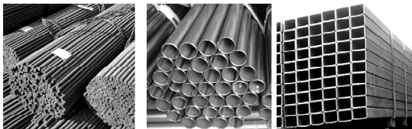
Fig. 1. Bundles of various types of long elements: bars, pipes and rectangular sections
