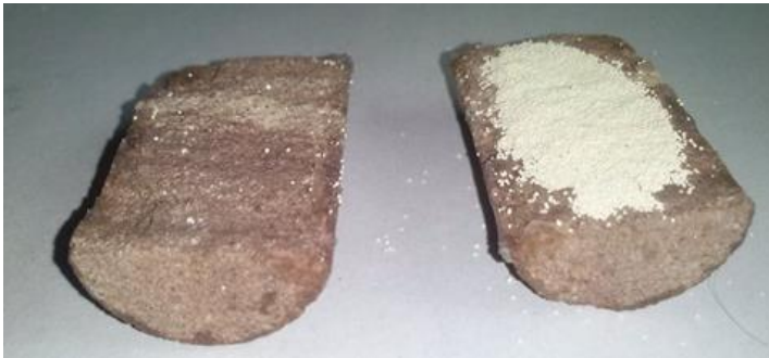
Fig. 6. Photo of the sandstone core filled with CP sample before placement in the permeability setup
