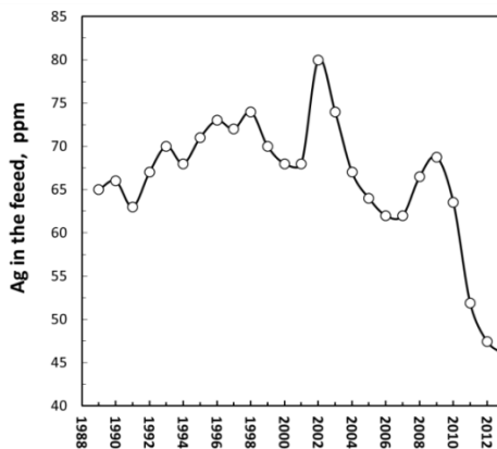
Fig. 2. Decreasing content of Ag in the feed of Lubin Concentrator (after Kukuc and Bazan, 2013)
