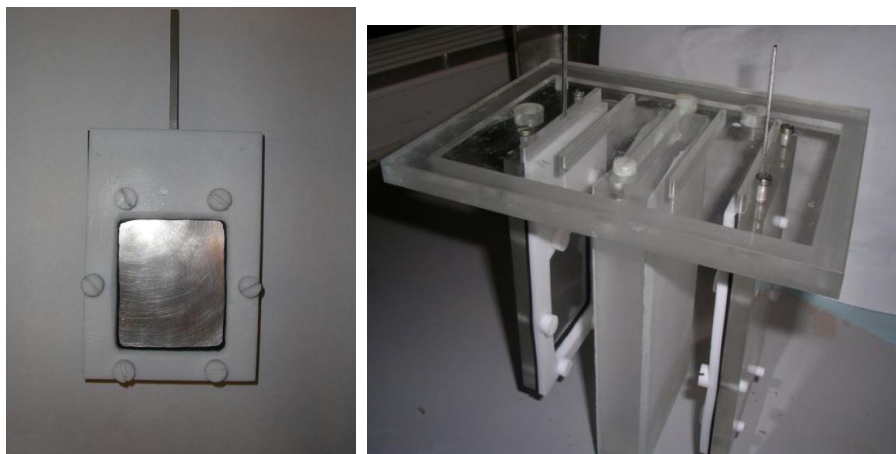
Fig. 1. Left: stainless steel blank in teflon mask. Right: cell cover lid attached with two steel blank cathodes
