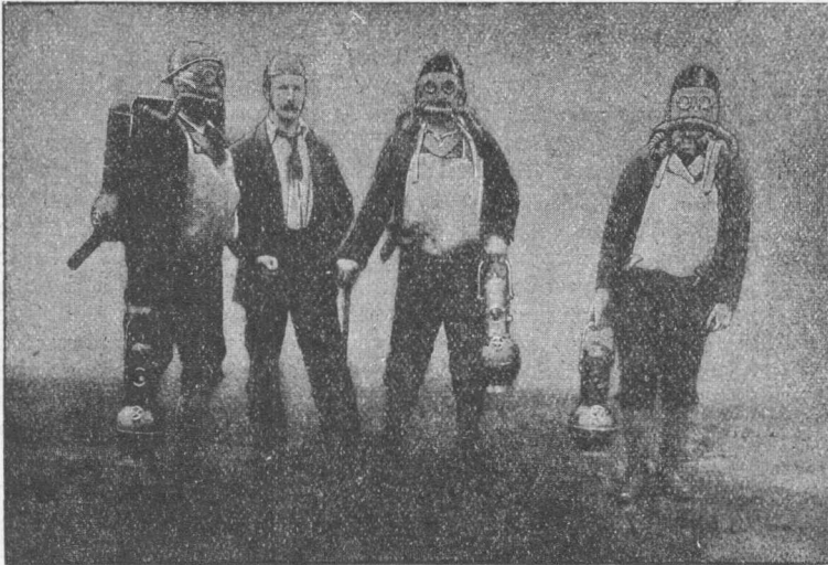
FIG. 1.—Henry A. Fleuss and group of miners, equipped with earliest Fleuss apparatus and oxygen lamps. Seaham Colliery, 1881.
