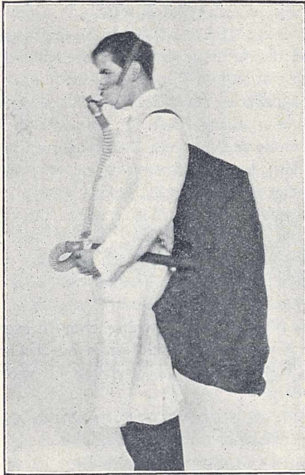
FIG. 2.—Bag, pipe, tap, valves, and mouthpiece used to investigate the gaseous exchanges of man during running.
