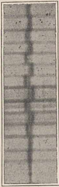
FIG. 6.—The Zeeman triplet \lambda 6173 in the sun-spot spectrum. Photographed in the second order spectrum of the 75-foot spectrograph of the Mount Wilson 150-foot tower telescope. The polarity of the spot is determined by the transmission of the red or violet component of the triplet by the "marked strip" of the compound quarter-wave plate.
