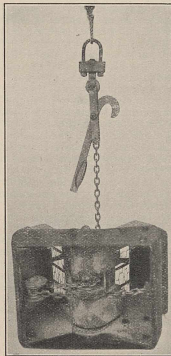
FIG. 1.—Petersen Grab modified to cut into a rectangular surface of the sea-bottom and to ensure partial protection of the gap present during closure. (From a photo by Mr. A. J. Smith.)
