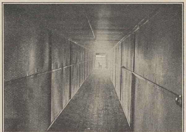
FIG. 2.—Insulated tunnel for the horizontal testing of mirrors and objectives.
