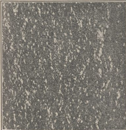
FIG. 2.—Photo-micrograph of surface of flint fractured by thermal agency. ( \times 100 .)
