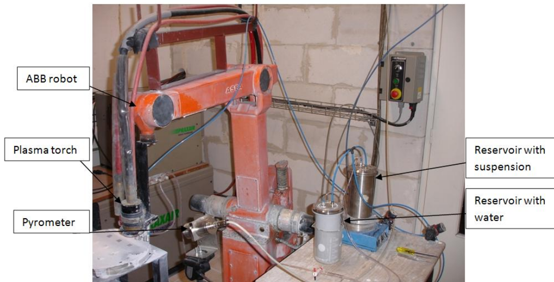
Figure 3.9 Plasma spraying installation.
