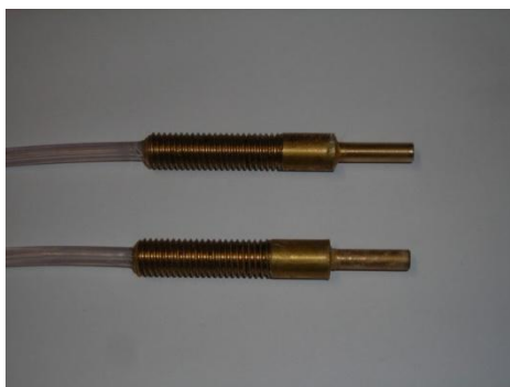
Figure 3.7 View of continuous stream nozzles.
