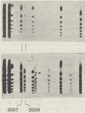
FIG. 1. Fabry-Perot patterns of the aluminium arc lines 3057A. and 3050A. Above, 10 mm. plate separation; below, 12 mm. plate separation.
