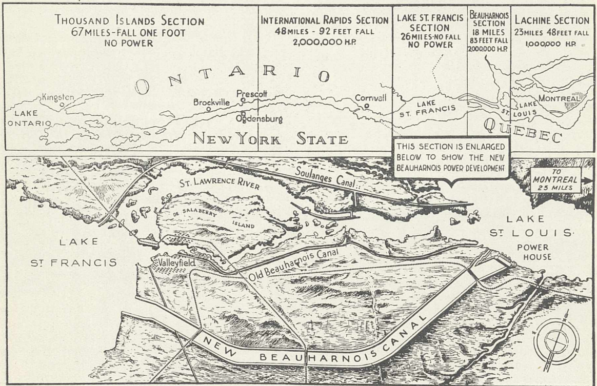
FIG. 3. Sketch map of Beauharnois hydro-electric power development.
