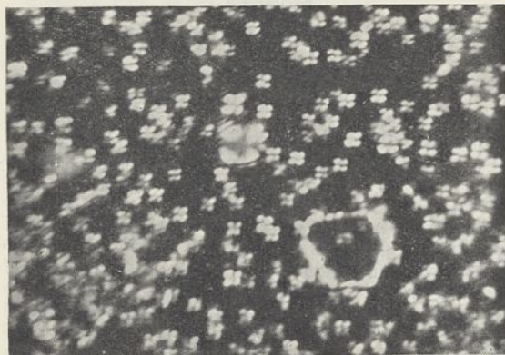
FIG. 1. Spherulitic particles on a silver film, and a large cubic crystal with birefringent edges. The spherulitic particles on the top of this crystal itself are due to a second sputtering, and subsequent heating. ( \times 2,000 .)
