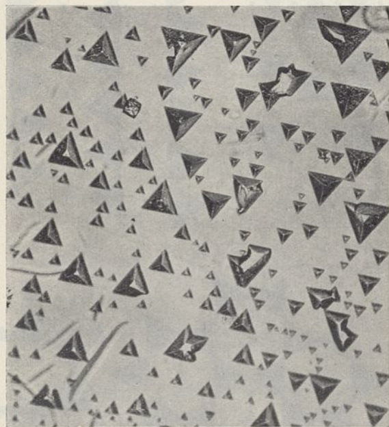
FIG. 3. The growth of ammonium iodide on mica (lepidolite). A sub-microscopic step on the mica sheet separates the two areas where the ammonium iodide crystals point in opposite directions. Each area is a true plane to within a single molecule. ( \times 80 .) Photograph by Mr. C. W. Bunn, Imperial Chemical Industries, Research Laboratory, Northwich.
