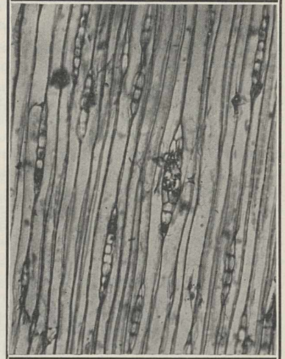
FIG. 2.—Photomicrograph of strip similar to that in Fig. 1, taken from spruce. Note the great length of the cells. \times 133 .
