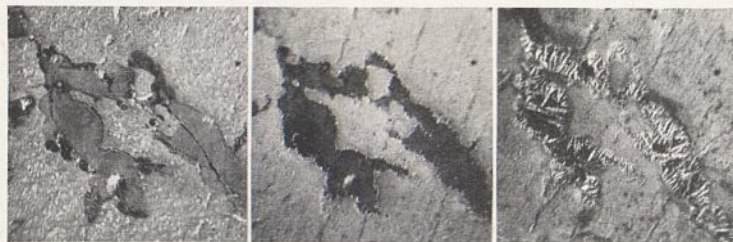
A B C MICROGRAPHS OF LEAD CONTAINING INCLUSIONS OF LITHARGE ( \times 25 ).
