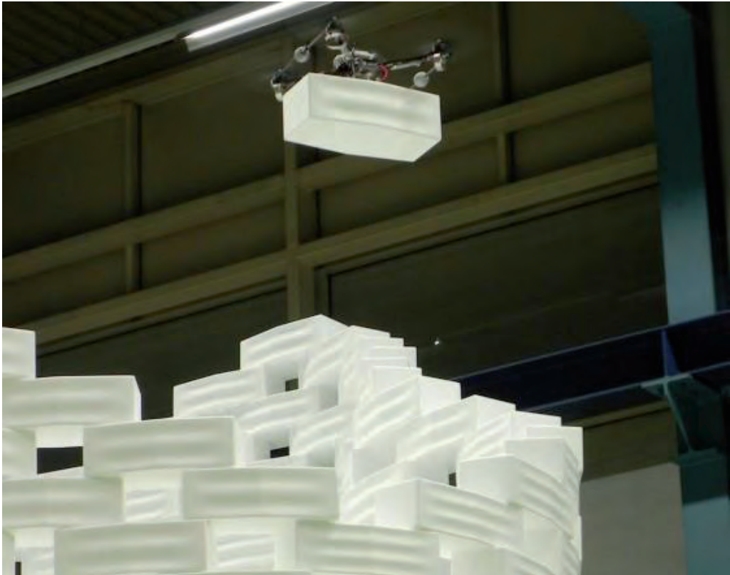
Fig. 3. One Quadrocopter from the project “Flight-Assembled Architecture” is setting a brick module in the process of assembling a tower (by Gramazio, Kohler, D’Andrea, ETH Zürich).
