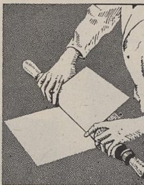
'Kodak' Transfer Sensitising paper is cemented to the lacquered metal
