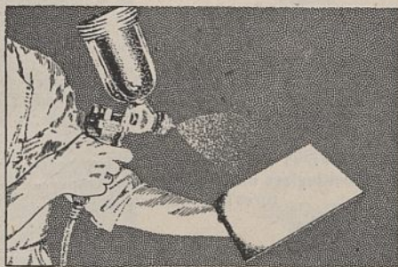
'Kodak' T.S. Lacquer is applied to the metal —in ordinary lighting —and allowed to dry
