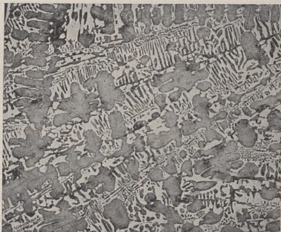
Hyper-eutectic white iron showing pearlite (half-tone) and cementite (white)
