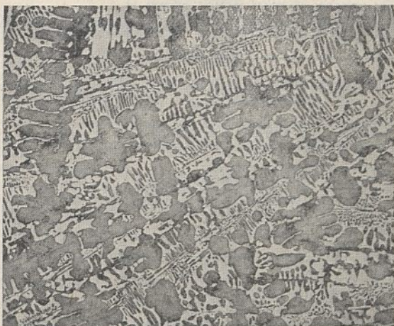
Hypo-eutectic white iron showing pearlite (half-tone) and cementite (white)
