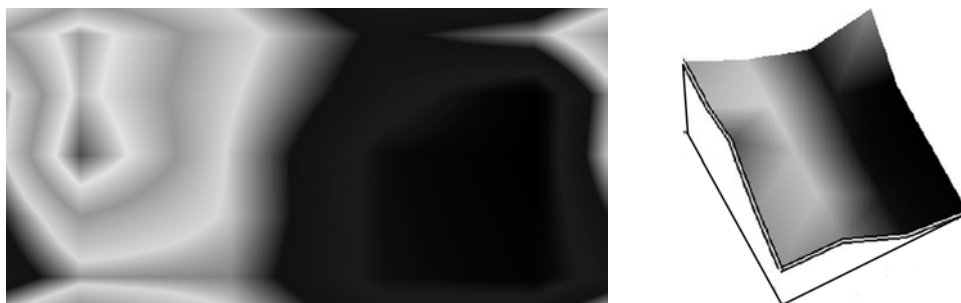
Fig. 5. Raman mapping of RBM band. Comparison between a top view (left panel) and a 3D view (right panel). The grayscale indicates the intensities of the band. Laser excitation 785 nm
