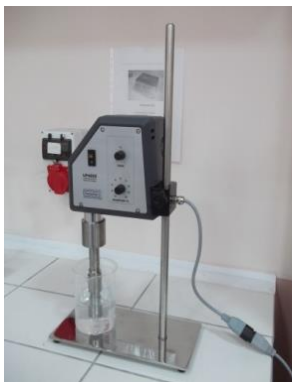
Fig. 2. Ultrasonic processor used
