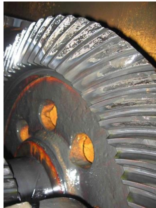
Fig. 5. Heavily effected/destroyed gear teeth, and colours heat tint
