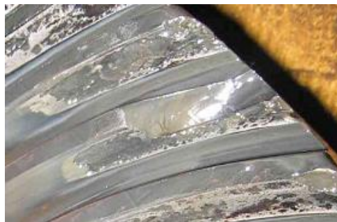
Fig. 6. View of damaged gear, fatigue fracture area with beach marks, brittle fracture area
