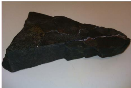
Fig. 2. Copper-bearing shale from T240b heading in area of R-VIII shaft pillar of Rudna Copper Mine (Poland)
