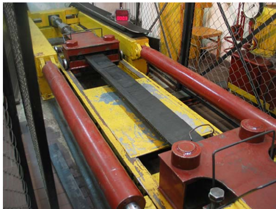
Fig. 2. Tensile testing machine ZP-40 for belt joints
