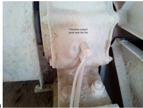
Fig. 3. a) Fan control equipment, b) a sensor control point near the Fan
