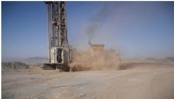
Fig. 2. Ingersoll-Rand T4BH Drill Rig in the mine
