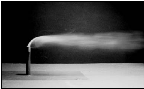
Fig. 3. Free streamline from free-standing chimney; u_H = 1.0 m/s
