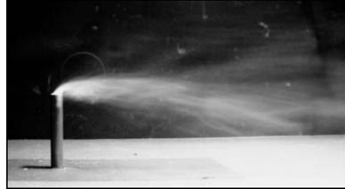
Fig. 10. Disturbed fume flow; u_H = 1.0 m/s; x_s = 9.5 H_B
