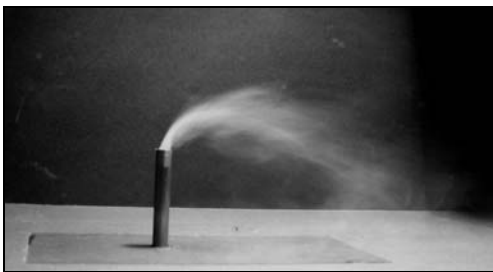
Fig. 9. Disturbed fume flow; u_H = 1.0 m/s; x_s = 6 H_B
