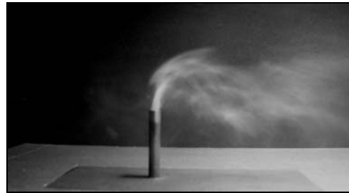
Fig. 8. Disturbed fume flow; u_H = 1.0 m/s; x_s = 4 H_B
