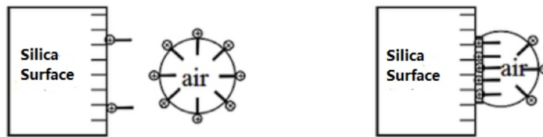
Fig. 9. Illustration of DDA molecules transferred to the quartz surface during bubble attachment
