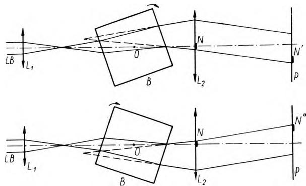
Fig. 1. Operation of a transparent four-wall block in a convergence beam
