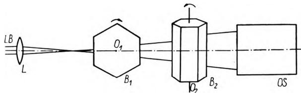
Fig. 2. Experimental device for coherent noise elimination in optical systems with laser illumination
