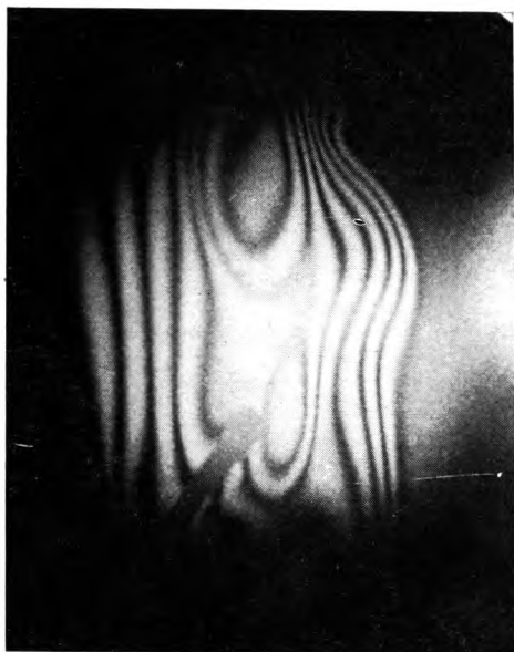
Fig. 4. An interferogram of the match flame
