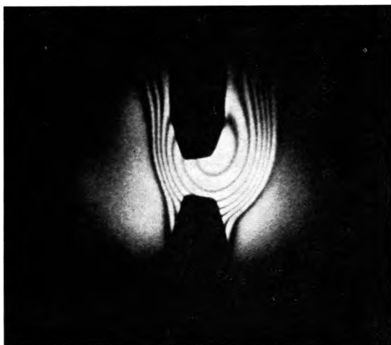
Fig. 5. An interferogram of the electrical arc
